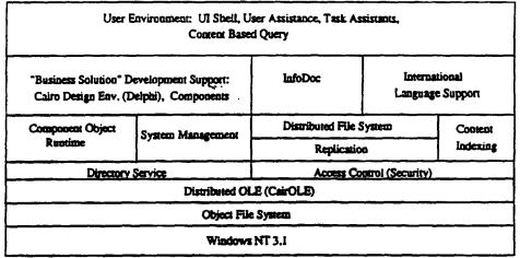
Figure 1. System Structure.
